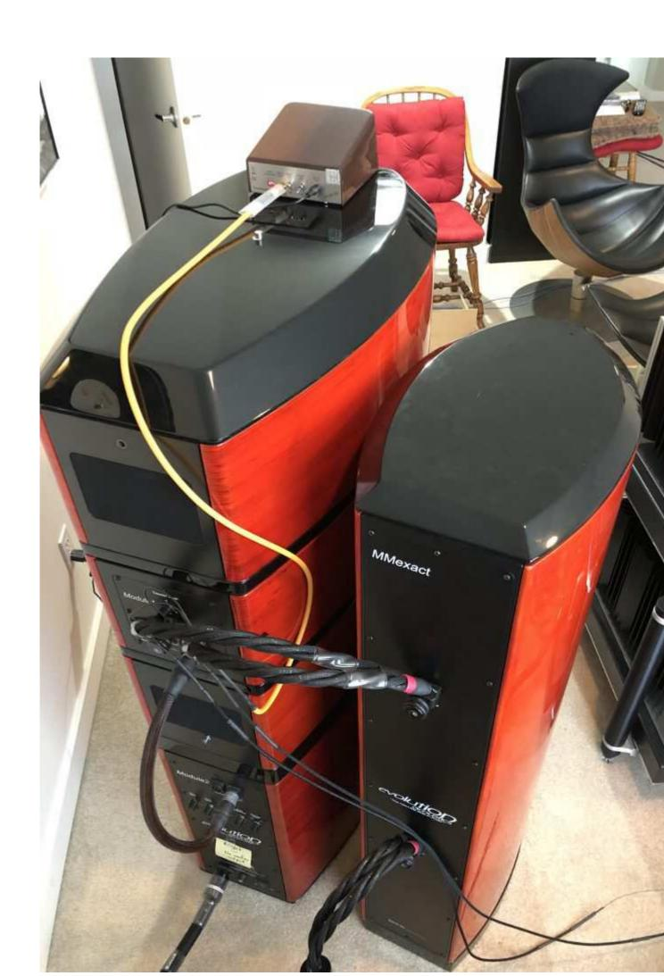
Rear view of The Extender resting on top of the Evolution Acoustics MM2 with EXACT External Crossover. The yellow cable is the van den Hul signal cable for The Extender. The large twisted cables are the Synergistic Research Galileo UEF; the thin black cables are the Synergistic Research wires for their Active Ground SE system.
